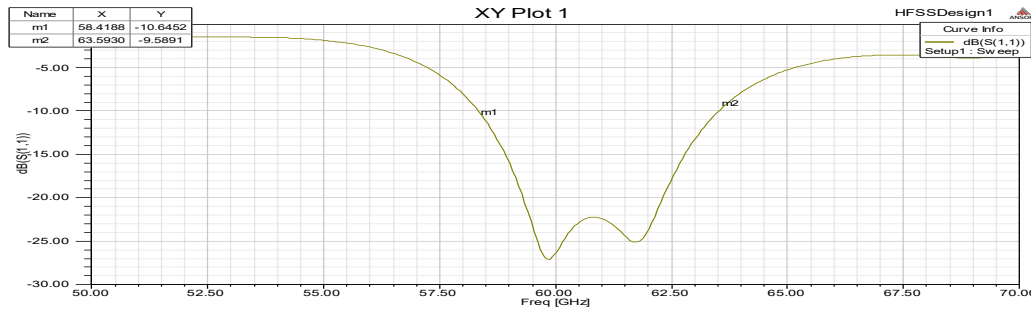
Figure 4.2. Return loss plot of single patch antenna
